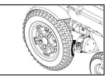
Figure 9. Drive Mode (Drive Engaged) - Hammer and H2 Motors
