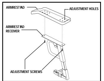
Figure 16. Armrest Pad Position Adjustment
