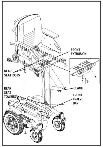
Figure 12. Seat Installation
