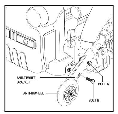
Figure 20. Anti-Tip Wheel Assembly
