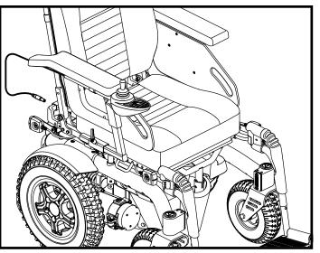
Figure 13. Controller Cable Routing (Rear Electrical System Shown)
