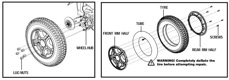
Figure 22. The R-4000 Series Drive Wheel
