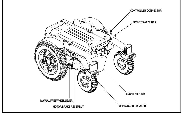
Figure 6. The Quantum R-4000 Series Power Base
