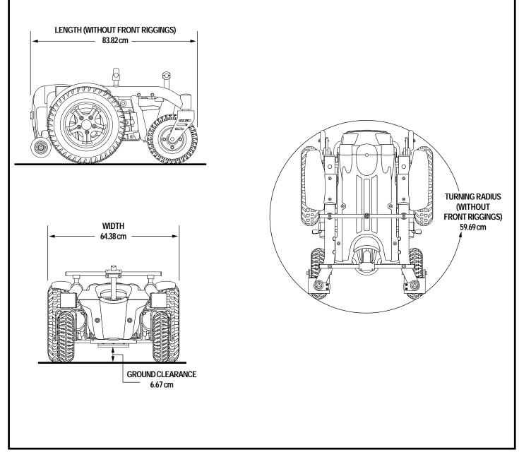
Figure 25. Quantum R-4000 Series Dimensions and Ground Clearance
