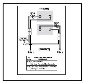
Figure 24. Battery Wiring Diagram
