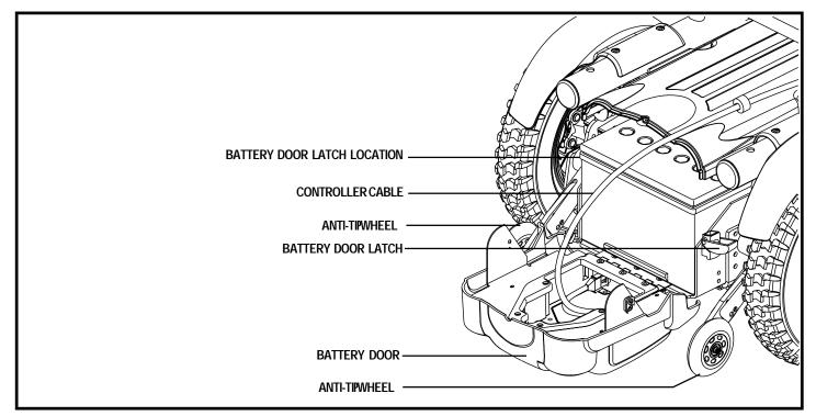
Figure 7. The Quantum R-4000 Series Power Base (Rear View - Battery Door Down)
