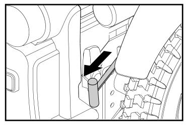
Figure 10. Freewheel Mode (Drive Disengaged) - Glide Motor Figure 11. Drive Mode (Drive Engaged) - Glide Motor
