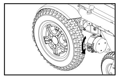
Figure 8. Freewheel Mode (Drive Disengaged) - Hammer and H2 Motors
